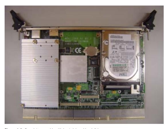
$\textbf{Figure 1-5}: \ \textbf{Complete assembly with heat sink and hard disk}$
